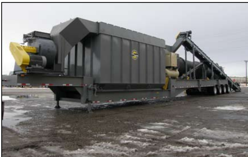
HRB-384 dryer mounted baghouse for lower transportation costs.
