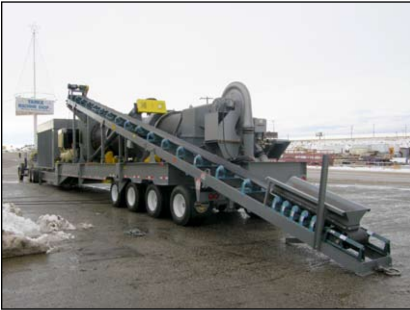
Aggregate scale conveyor is mounted to the dryer frame for lower transportation costs.
