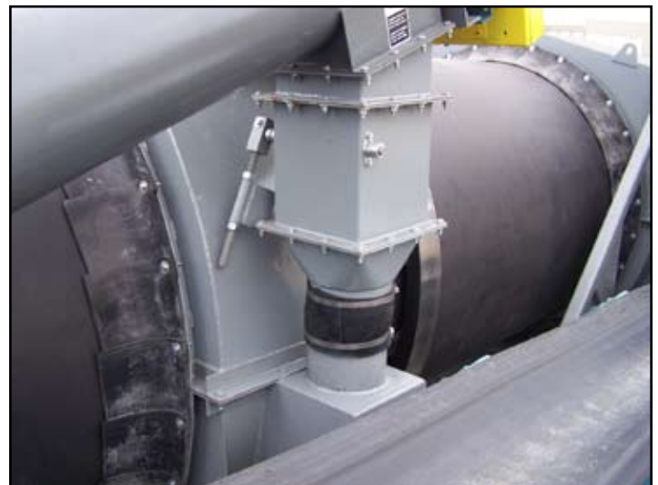
Dust tipple valve feeds the dust back into the mixer from the knockout box and baghouse.
