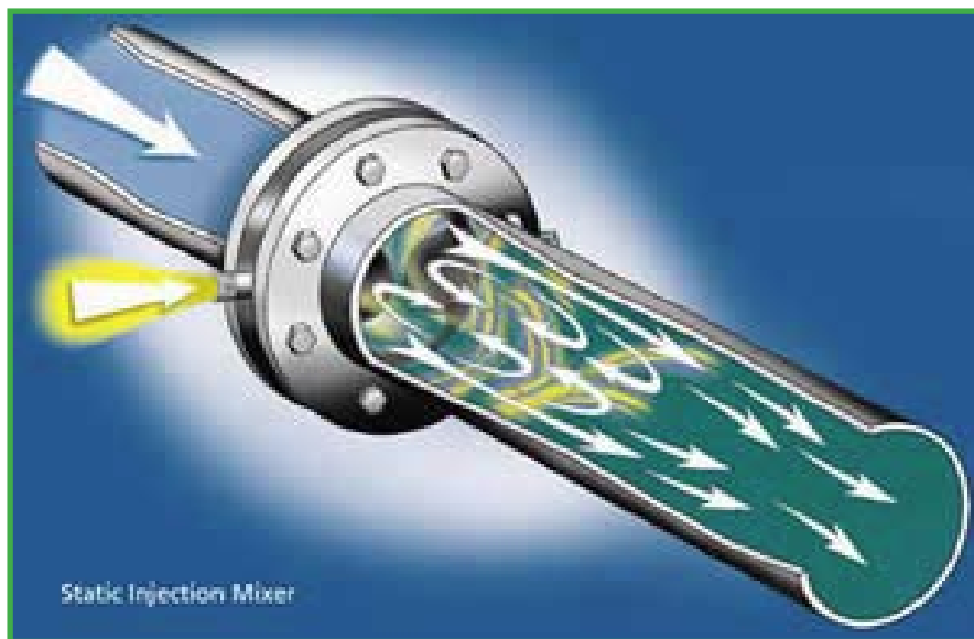
Eco-Foam II Mixer showing the reverse flow regions.
