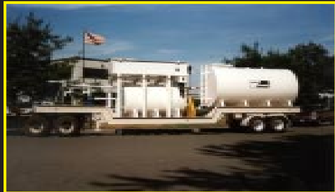
Lime/Slurry Mixing Trailer
